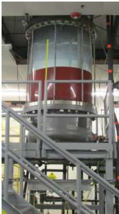
Fig.13. Full Scale IX Test Column Containing Resin
