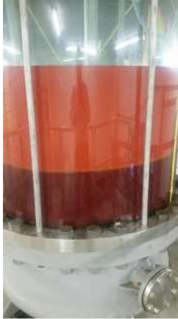
Fig.15. sRF Resin Part Way Through Elution Process
